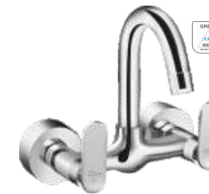
F1018501 Sink mixer (wall mounted) with 150 mm (6'') long swivel spout, connecting legs and wall flanges
