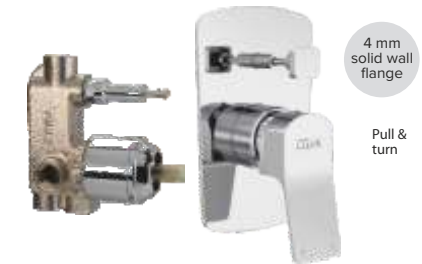
5 - Way (3 inlets + 2 outlets) single lever concealed diverter Exposed Part without tipton & sleeve Concealed Part with sleeve Exposed Part F1021711 Concealed Part F4020101
