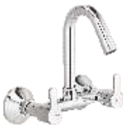
F1015501 Sink mixer (wall mounted) with 190 mm (7.5") long swivel spout, connecting legs and wall flanges
