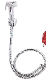
F8030105AB Health Faucet ABS body with 1 meter SS braided connection pipe
