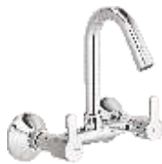
F1015501 Sink mixer (wall mounted) with 190 mm (7.5") long swivel spout, connecting legs and wall flanges ₹ 4,560
