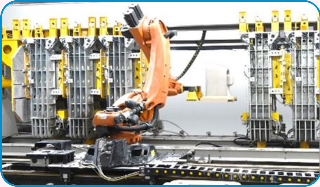
Sanitaryware Robotic Pressure Casting:
