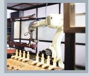
Faucet Robotic Surface Grinding - Helps in uniform coat of chromium plating that will lead to surface endurance
