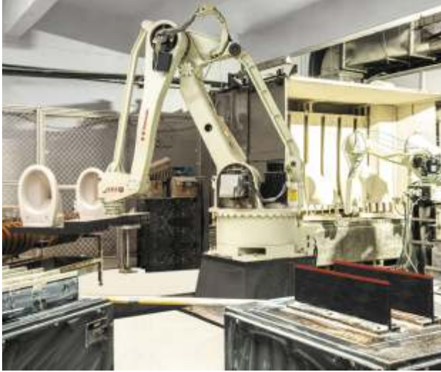
Sanitaryware Robotic Glazing For uniform glazing ensuring smooth surface
